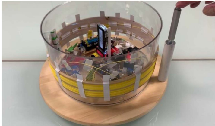
Video 4. Fiber ring interferometer rotated in both directions, starting from the value 001 displayed at rest When rotated, the displayed value increases in the same manner in both directions. (An animation of this figure is available in the online article .)
