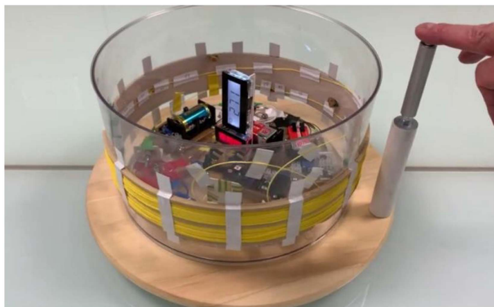
Video 5. Fiber ring interferometer rotated in both directions, starting from the value 249 displayed at rest In this example, when rotated, the displayed value increases in one direction and decreases in the other. (An animation of this figure is available in the online article .)
