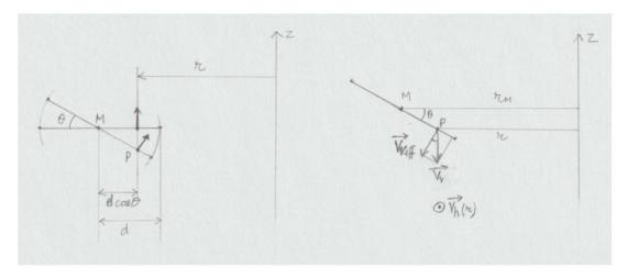
On the diagrams representing the horizontal wing and the same wing inclined at an angle q, we see that the modifications which affect the quantities entering into the calculations are as follows:
