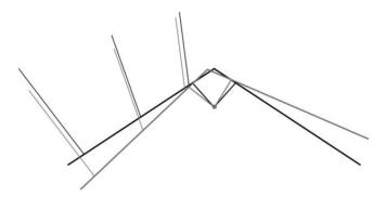
When a roll rotation is imposed on the IAP, each line is pulled a certain length on one side and released a certain length on the other side; and for the same line, these lengths increase continuously from column 1 to column 3 (and column 4 of the stabilizer lines, if there is one).
