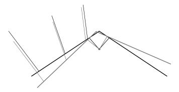
When a roll rotation is imposed on the iap, each line is pulled a certain length on one side and released a certain length on the other side; and for the same line, these lengths increase continuously from column 1 to column 3 (and column 4 of the stabilizer lines, if any).
