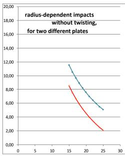
Increasing the pitch has the effect of increasing the different impacts along the span by the same amount (shifting the curve upwards).
